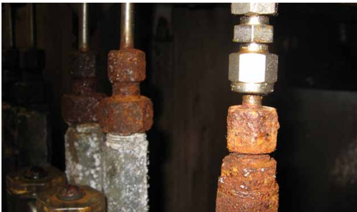
Galvanic reaction created by mixing different body & nut materials.
