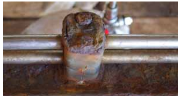
Crevice corrosion between the tube/tube trap interface.
